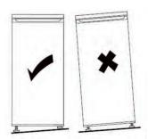
When the refrigerator stays in the packing box, plastic feet are in tightened state. After carrying it out from the packing box for placement, please make sure to adjust two front plastic feet until the height is suitable; just adjust two plastic feet with a wrench or directly by hand.
