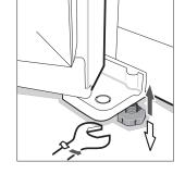
When moving the refrigerator, adjust plastic feet counterclockwise to keep them off the ground, and then push the refrigerator gently to move it.
