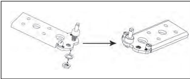
8. Transfer the lower door to the property position. Replace both adjustable feet.
