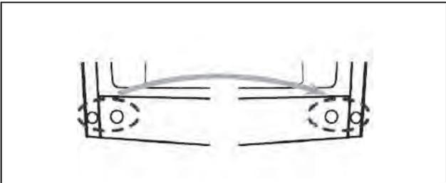
10. Make the middle hinge reverse the direction 180°, then transfer it to the left property position. Make the middle hinge pin in the upper hole of the lower door, then tighten the bolts.
