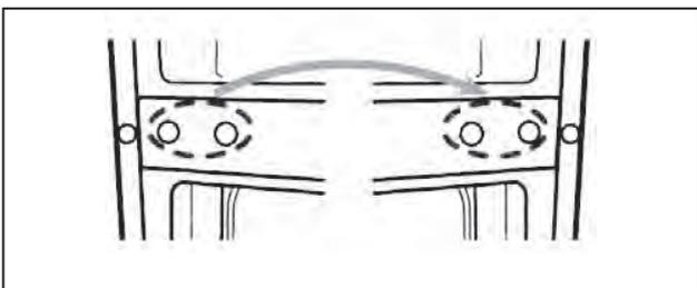
**6. Unscrew bottom hinge. Then remove the adjustable feet from both.**
