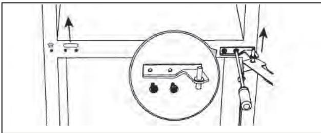
**4. Move shaft sleeve and pinhole plug from left side to right side.**
