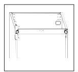
**12.** Remove hinge assist from bottom of upper and lower doors, then take new hinge assist piece form accessary bag and install them to the left side.
