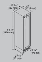
Stated minimum height dimensions include when the leveled feet are fully inserted.
