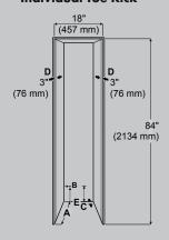
Cabinet depth frameless installation style = 25" (635 mm) Cabinet depth inset installation style = 25" (635 mm) + panel thickness
