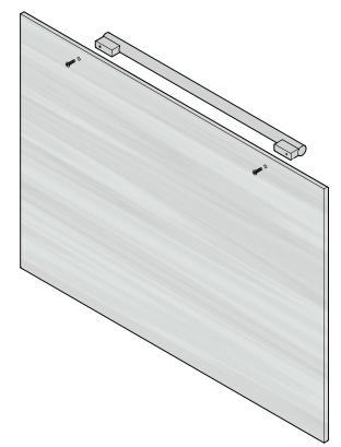
Only use countersunk screws for handle mounting.
