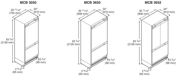
Stated minimum height dimensions include when the levelled feet are fully inserted. Width will increase by 1/4" (6.5 mm) when mounting strips are installed.
