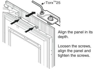
Loosen the screws, align the panel and tighten the screws.
