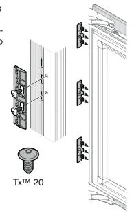
Fasten the panel through the bottom attachment bracket with two screws  $4 \times 14$ .
