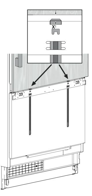
*IMPORTANT* Now install the door handles as the attachment bracket will cover the mounting holes.
