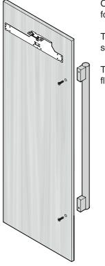
Only use countersunk screws for handle mounting.
