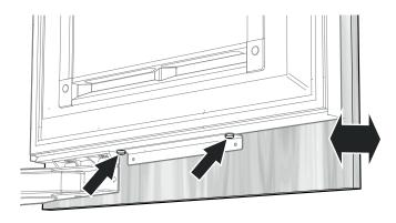
Insert the panel supports into the support strips between panel and appliance door and screw into place with two screws M6 x 12 each.
