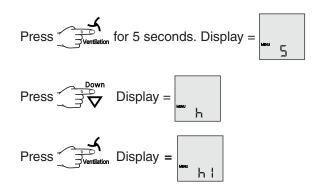
Use buttons Up and Down to select the desired setting.
