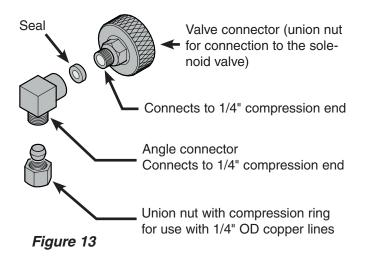
The connection to the valve connector can be done with or without the angle connector, as required.
