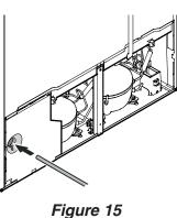
3. Move the power supply line to the area of the electrical outlet.
