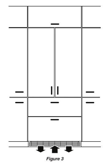
It is important to use the provided cover grille for the ventilation opening. This opening must not be covered with a cabinet base.
