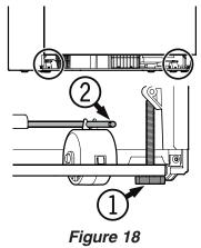
To prevent the appliance from tipping forward the leveling feet (1) (Figure 19) must have contact with the floor.
