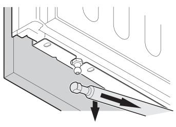
7. Dismantle the lower attachment bracket from the refrigerator door. Align the bracket to the lines on the refrigerator door panel. *(Figure 28)*.
