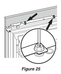
To make it possible to fasten the refrigerator panel at the bottom the soft-stop cylinder must be dismantled.
