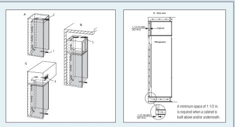
This is a fully integrated refrigerator-freezer which means that it is fully enclosed by a kitchen cabinet. This type of cabinet must be carefully constructed using the correct dimensions and it must provide suitable ventilation to ensure proper appliance operation.
