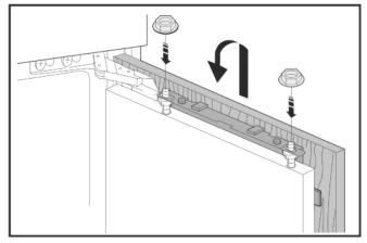
Fig. 44Attach the unit door and loosely screw the lock nuts onto the adjusting bolts.
