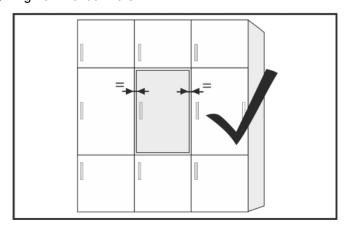
Fig. 46► Check the gap between the door and the surrounding unit doors
