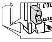
▶ Undo the screw and remove the spacers.
