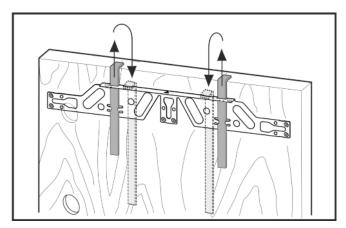
Fig. 42Remove the fitting aids, turn round and insert into the adjacent opening.
