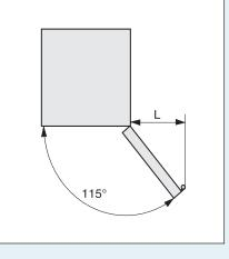
G. 21-5/8" (550 mm) H. 1-5/8" (40 mm) J. 27-3/8" (695 mm) K. 24-3/4" (629 mm) L. max. 3/4" (19 mm) M. 9-21/32" (245 mm)
