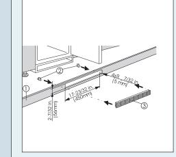
Ventilation through the cabinet base at the bottom can be achieved by installing the provided ventilation grille (3) or via a ventilation opening of at least 31 in.<sup>2</sup> (200 cm<sup>2</sup>).
