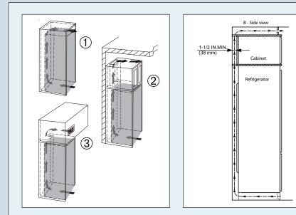
Do not restrict the air flow. The opening can either be directly over the appliance  $\oplus$ , above the cabinet and below the ceiling @ or through a vent installed in a soffit @.
