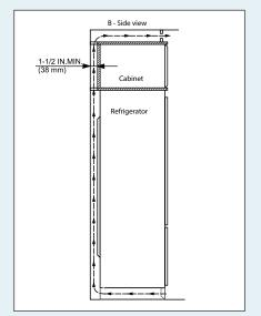
Do not restrict the air flow. The opening can either be directly over the appliance  $\odot$ , above the cabinet and below the ceiling @ or through a vent installed in a soffit @.
