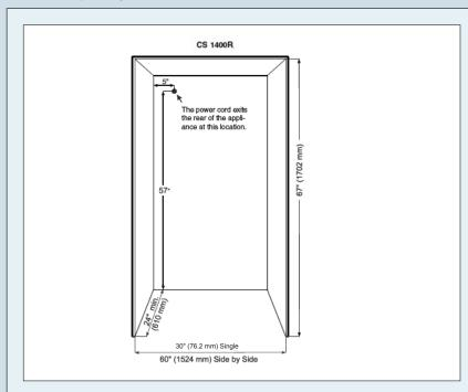
The appliance can be used freestanding or semi built-in. If semi built-in, consider the cabinet opening dimensions.
