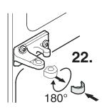
**22.** Remove hinge bushing, turn through 180° and re-fit.
