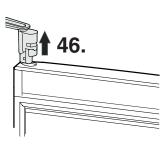
**46.** Using a screwdriver, push out the hinge from underneath and remove it from the door .
