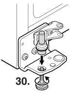
30. Tilt appliance slightly backwards, insert pin and attach using the adjustable foot.
