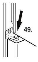
**49.** Suspend top door on hinge pin. For this, the door must be open at least 90°.
