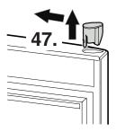
**47.** Using a screwdriver, push out the plug from underneath and transfer it to the opposite side.
