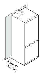
Clearance on the back must be 2 inch (51 mm).
