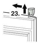
**23.** Using a screwdriver, push out the plug and transfer it to the opposite side.
