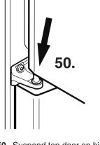
Suspend top door on hinge pin. For this, the door must be open at least 90°.
