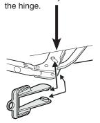
**IMPORTANT** The two knobs on the safety bracket must be fully inserted into the marked openings on the hinge.
