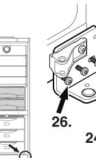
24. Tilt appliance slightly backwards and unscrew the adjustable foot.
