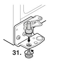
**31.** Tilt appliance slightly backwards, insert pin and attach using the adjustable foot.
