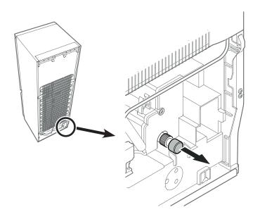
5. Screw the adapter onto the solenoid valve.
