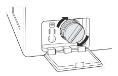
**8** Close the drain pump filter cover.
