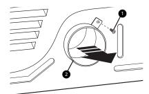
2 Press the tabs on the knockout ③ and carefully remove the knockout for the desired vent opening. (Right-side venting is not available on gas models.) Press the adapter duct ④ onto the blower housing and secure to the base of the dryer as shown.
