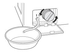
**5** Clean the pump filter and opening.
