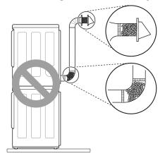
Make sure the ductwork is not crushed or restricted.
