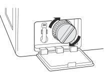
**8** Close the drain pump filter cover.
