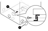
3 Preassemble a 4" (10 cm) elbow (5) to the next 4" (10 cm) duct section, and secure all joints with duct tape. Be sure that the male end of the elbow faces AWAY from the dryer. Insert the elbow/duct assembly through the side opening and press it onto the adapter duct. Secure it in place with duct tape. Be sure that the male end of the duct protrudes 1 1/2" (3.8 cm) to connect the remaining ductwork. Attach the cover plate (5) to the back of the dryer with the included screw.
