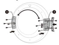
On the appliance cabint, unscrew 2 screws and remove the door catch **⑤**. Reassemble it on the opposite side of the door.
