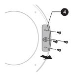
Swap the position of the hinge assembly 3 and the door latch assembly 4 and reassemble. Refer to steps 2 and 3 for the location and number of screws when reassembling.
