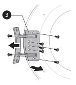
Remove the 3 screws from the door latch assembly 4 which is mounted between the door and the hinge assembly. Remove the screw in the door latch.
