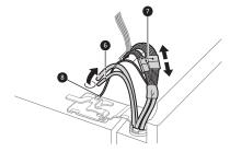
Rotate the hinge lever **9** counterclockwise. Lift the top hinge **1** free of the hinge lever latch **①**.
