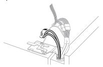
Hold the water supply connection and gently push in the collet **4** to connect the water supply lines as shown. Insert the tube at least 5/8 inch (15 mm) into the connector. Insert the clip on the joint to fasten the tubes in place.
