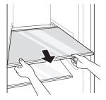
**3** To assemble, tilt the front of the shelf up and guide the shelf into the slots at a desired height, keeping shelf holder down.
