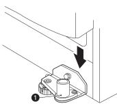
2 Fit the hinge 2 over the hinge lever latch 3 and slot it into place. Rotate the lever 4 counterclockwise to secure the hinge.
