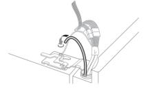
5 Hold the water supply connection and gently push in the collet ④ to connect the water supply line as shown. Insert the tube at least 5/8 inch (15 mm) into the connector. Insert the clip on the joint to fasten the tube in place.
