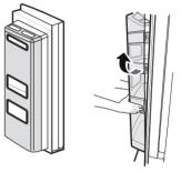
**2** To remove the baskets, lift up and pull out.
