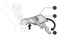
**3** Lift the door from the middle hinge pin and remove the door.
