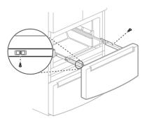
**3** Grip both sides of the drawer and pull it up to remove it from the rails.
