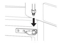
2 Fit the hinge ① over the hinge lever latch ② and slot it into place. Rotate the lever ③ counterclockwise to secure the hinge.
