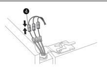
**3** Connect all the wire harnesses and the ground screw.
