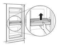
**2** To lower the bin, press the side levers up at the same time and move the bin down until it clicks into place.
