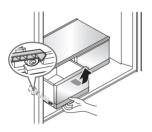
**2** Lift the front of the cover with one hand and support underneath the cover with the other hand.
