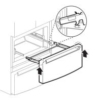
**3** Lower the door into its final position and insert the screws in the rails on both sides.
