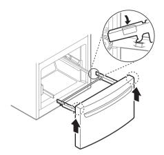
**3** Lower the door into its final position and insert the screws in the rails on both sides.
