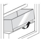
**2** To assemble drawers, slightly tilt up the front, insert into the frame and push back into place.
