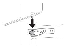
Fit the hinge **1** over the hinge lever latch **2** and slot it into place. Rotate the lever 3 clockwise and fasten the hinge.
