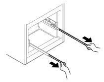
**2** Grasp the drawer on each side and hook the drawer supports into the rail tabs located on both sides.
