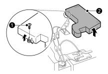
2 Detach all the wire harnesses **3**. Unscrew the ground wire **4**. Remove the cover.
