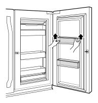
**2** To replace the door bins, slide the door bin in above the desired support and push down until it snaps into place.
