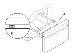
Grip both sides of the drawer and pull it up to remove it from the rails.
