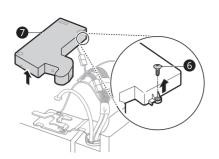
Remove the cover and pull out the tube 8. Disconnect all wire harnesses 9. Unscrew the ground wire **10**.
