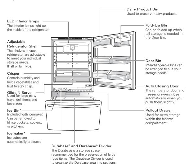
It can be adjusted from side to side to accommodate items of different sizes.
