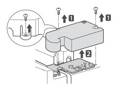
Using a 10mm or 13/32 in. socket wrench, remove the three bolts and lift off the top hinge. Set parts aside.
