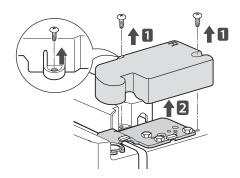
Remove the three bolts using a 10mm or 13/32-inch socket wrench and lift off the top hinge. Set parts aside.
