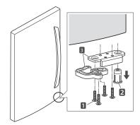
Reinstall the hinge pin brackets 1, screws 2 and hinge pin insert 3 on the bottom left side of the door.
