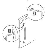
3 Carefully loosen the plug button with your fingers. The buttons can be unscrewed with the fingers by rotating them counter-clockwise and continuing until they loosen and fall out The buttons were installed without pressure, and for this reason, they can be unscrewed using your index finger, thumb or both. Install the plug buttons 5 on the left side.
