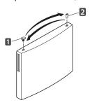
13 Re move the decorative caps on the bottom of the refrigerator housing. You will need these holes for the bottom hinge.
