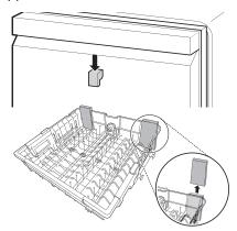
Press the tab to remove the cable tie by hand.
