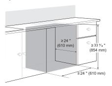
To allow for proper clearance of plumbing and electrical, use the template included with the literature to determine the clearance on the side of the cabinet where the cabinet meets the back wall. Using a 2 1/2" diameter hole saw, drill a hole in the target area as shown on the template.
