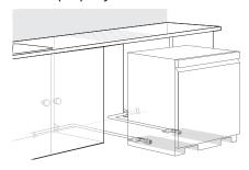
Smooth out or pad the edges of the hole drilled for the water supply to avoid damaging the drain hose.
