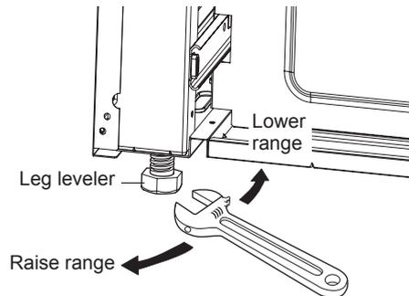
Use a level to check your adjustments. Place the level diagonally on the oven rack, and check each direction for level.
