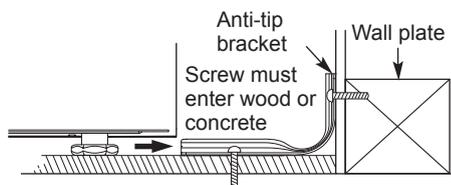
The anti-tip bracket is packaged with an installation template. The instructions include necessary information to complete the installation. Read and follow the range installation instruction sheet.
