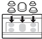
**Make sure that all grates are properly placed before using the burner.**
