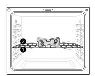
If the level doesn't show that the rack is level, adjust the leveling legs with a wrench.
