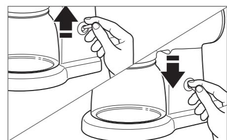
5. Flip the POWER switch up to turn on, and begin grinding your coffee. Flip the POWER switch down when you have ground the desired amount of coffee.
