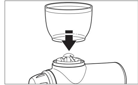
1. Make certain the Burr Grinder is unplugged. Attach the bean hopper to the top of the motor housing, turning clockwise until snug.
