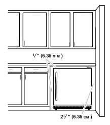
To ensure proper ventilation for your wine cellar, allow for a 1/" (6.35 mm) space on each side and at the top. When installing your wine cellar next to a fixed wall, leave  $2^1/$ " (6.35 cm) minimum clearance on the hinge side to allow for the door to swing open.
