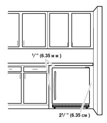
For the wine cellar to be flush with the front of the base cabinets, remove any baseboards or moldings from the rear of the opening. See "Opening Dimensions" later in this section.
