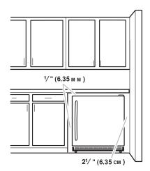
To ensure proper ventilation for your refrigerator, allow for a  $\frac{1}{1}$ " (6.35 mm) space on each side and at the top. When installing your refrigerator next to a fixed wall, leave  $\frac{21}{1}$ " (6.35 cm) minimum clearance on the hinge side to allow for the door to swing open.
