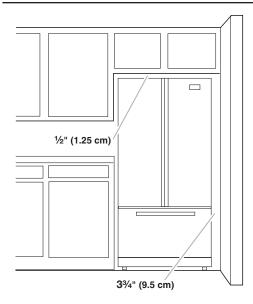
To ensure proper ventilation for your refrigerator, allow for a  $\frac{1}{2}$ " (1.25 cm) of space on each side and at the top. Allow for a 1" (2.54 cm) space behind the refrigerator. If your refrigerator has an ice maker, allow extra space at the back for the water line connections. When installing your refrigerator next to a fixed wall, leave a  $3\frac{3}{4}$ " (9.5 cm) minimum space between the refrigerator and wall to allow the door to swing open.
