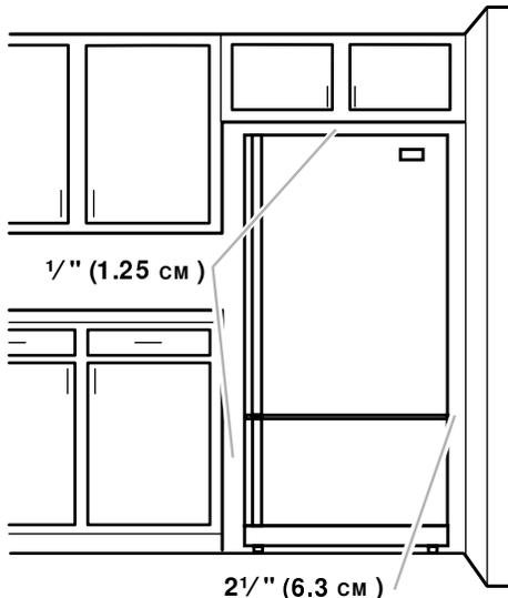
To ensure proper ventilation for your refrigerator, allow for a 1/2" (1.25 cm) space on each side and at the top. Allow at least 1" (2.54 cm) between back of cabinet and the wall. If your refrigerator has an ice maker, allow extra space at the back for the water line connections.
