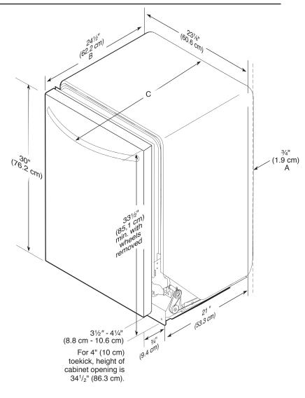
A. Insulation may be compressed (not used on all models).
