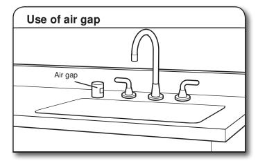
If required, the air gap should be installed in accordance with the air gap installation instructions. When you are connecting the air gap, a rubber hose (not provided) will be needed to connect to the waste tee or disposer inlet. Use 1/2" minimum I.D. drain line fittings.
