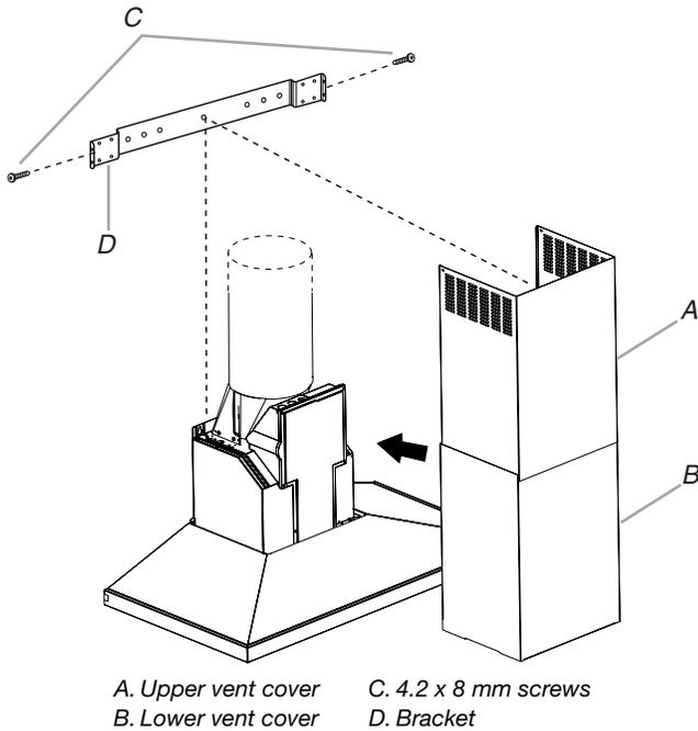
Secure the bottom of the duct with (2) 4.2 x 8 mm screws.
