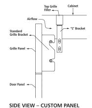
Attach the standard custom grille with the standard grille bracket provided with the refrigerator
