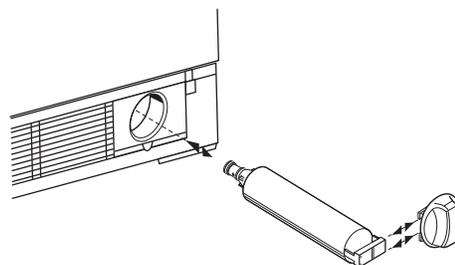
3. Take the new water filter out of its packaging and remove the cover from the O-rings.
