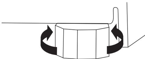
3. Remove the level and close the top drawer. Check the gap between the top of the drawer and the countertop. If the gap measures less than 3/8" (9.5 mm) minimum, turn all four leveling bolts equally to the left to raise the leveling legs (this will lower the appliance). Recheck the level.
