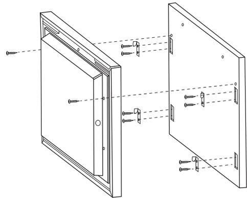
3. Gently pull back the gasket from the top corners of the door until you can see the screw that is behind the gasket. There is one screw on each side. It is not necessary to remove the gasket.
