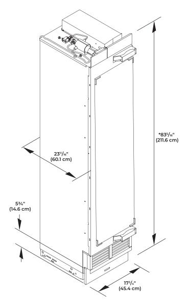
\*Add 1" (2.5 cm) to the height dimension when leveling legs are fully extended.
