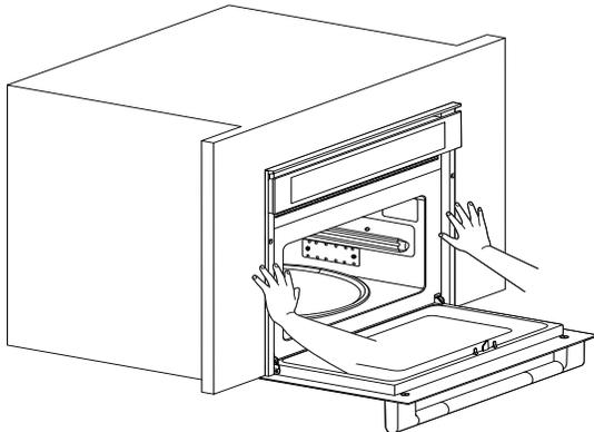
3. Securely fasten microwave oven to cabinet using two 3/4" (1.9 cm) flat-head screws provided. Insert the screws through holes in mounting rails. Do not overtighten screws.
