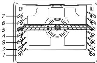
The oven has 7 positions for a flat rack, as shown in the previous illustration and the following table.
