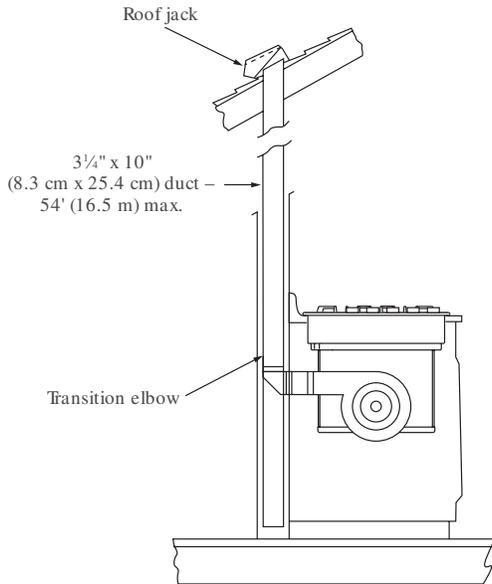
REAR DUCTING IN WALL TO ROOF
