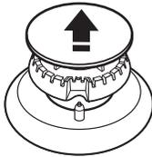
Remove burner cap and base.
