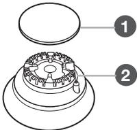
**IMPORTANT:** Do not obstruct the flow of combustion and ventilation air around the burner grate edges.
